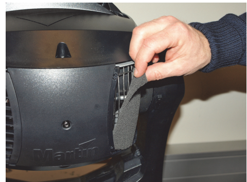
Figure 9: Removing head air filters
